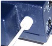
Insert one end of the fiber optic cable carefully into the fiber optic port on the encoder. Tighten the nut gently so that the cable won't slip out.
