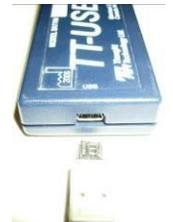
Insert the small connector of the USB cable into the USB port on the TT-USB interface device.
