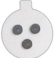
The image shows a circular EMG electrode with three dark spots. | <p><b>T3402M - Triode™ electrode</b>, with standard 2cm spacing of silver-silver chloride electrodes, backed with nickel plated brass snaps to prevent corrosion.</p> <p>The section <a href="#">Using the EMG sensor</a>, starting on page 15, describes how to set up EMG sensors with the correct electrodes and place them on an examinee.</p> |
