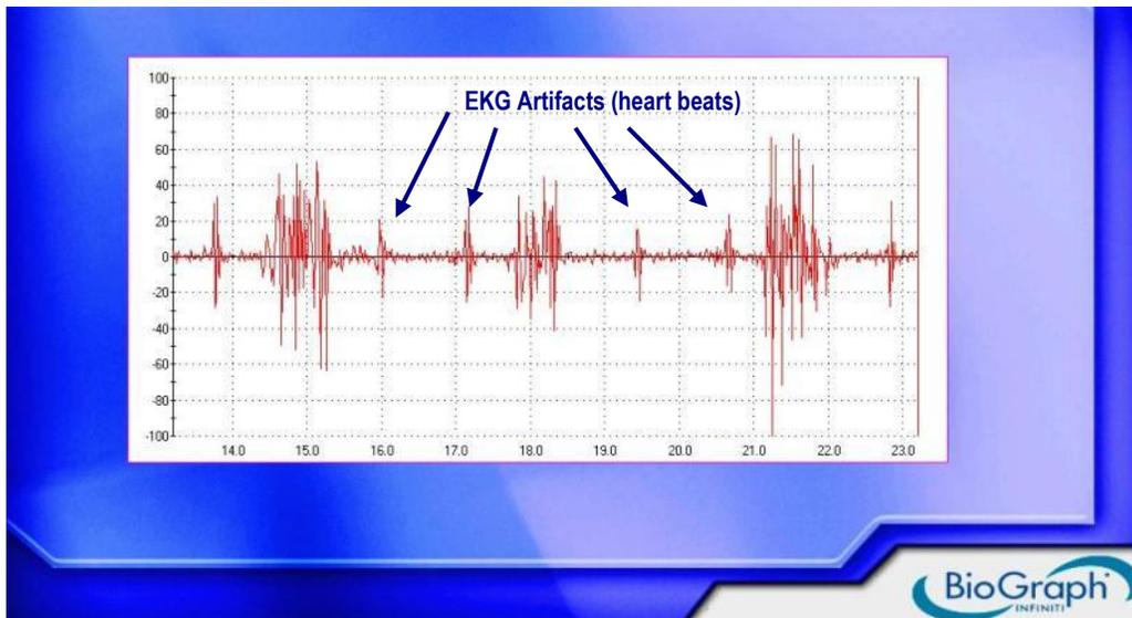
**Fig. 4. Raw EMG signal with EKG artifact**
