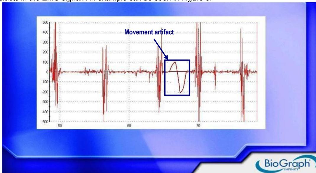
**Fig. 5. Raw EMG signal with movement artifact**
