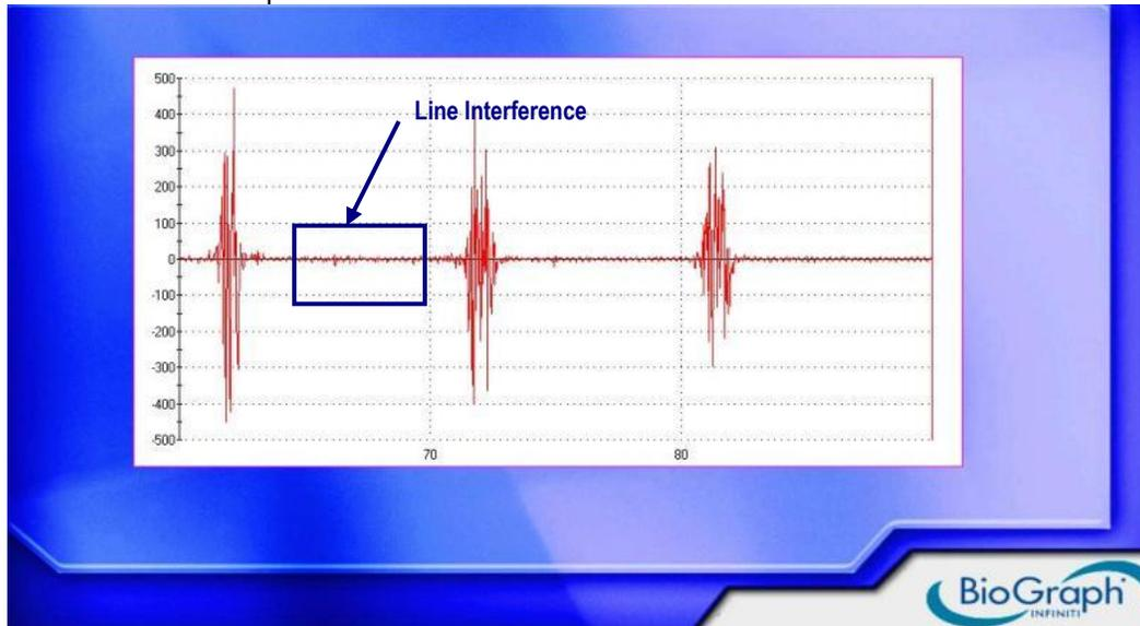
**Fig. 3. Raw EMG signal with line interference**
