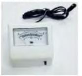
When monitoring with the reverse temperature sensor, the needle moves counter-clockwise with warming.
