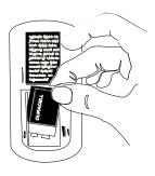
replace with a new battery. To prevent battery leakage, remove battery when the U-Control unit will not be used for one month or longer.
