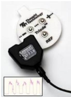
The MyoScan-Pro is a pre-amplified surface electromyography sensor for use on low sampling rate encoder inputs and designed to measure RMS SEMG.
