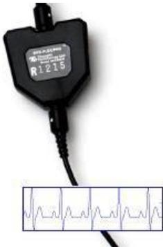
The EKG sensor is a pre-amplified electrocardiograph sensor, for directly measuring the heart's electrical activity. Connects via extender cables for a single channel hook up.
