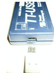
Insert the small connector of the USB cable into the USB port on the TT-USB interface device.
