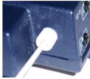
Insert one end of the fiber optic cable carefully into the fiber optic port on the encoder. Tighten the nut gently so that the cable won't slip out.
