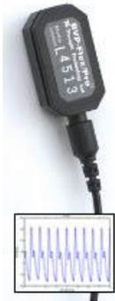
The HR/BVP sensor is a blood volume pulse detection sensor (otherwise known as a PPG sensor) housed in a small finger worn package, to measure heart rate (HR) and provide BVP amplitude, BVP waveform, HR and heart rate variability feedback.
