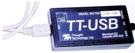
USB ports on a PC are generally located at the back of the base unit. You may also find a USB port at the front of your base unit; you can connect the other end of the USB cable to it. On a laptop, USB ports are usually located at the side or the back of the laptop. It is recommended to always use the same USB port for connecting the TT-USB to your computer.
