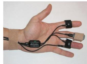
Close up view of temperature sensor and skin conductance finger strap.
