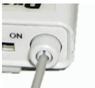
Insert one end of the fiber optic cable carefully into the fiber optic port on the encoder as far as it will go. Tighten the nut gently so that the cable won't slip out.
