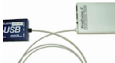
Do the same with the other end of the fiber optic cable and the fiber optic port of the TT-USB interface unit.
