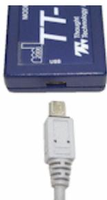
Insert the large connector of the USB cable into the USB port of your PC.
